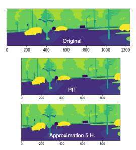
Figure 2. **Approximating PIT with homographies.** We show the original image (top), the PIT [13] correction (middle), and our approximation of PIT using 5 homographies. Note that 5 homographies are sufficient to closely match the PIT spherical correction.
