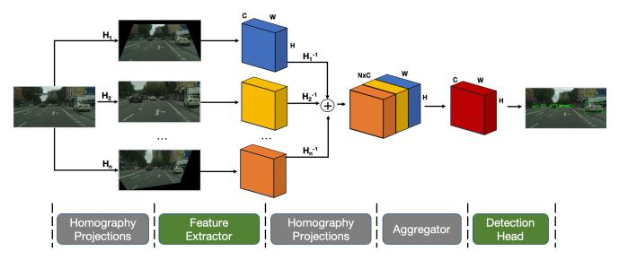
Figure 3. **Architecture**: The input image is first transformed by a set of trainable homographies. The feature maps extracted from the transformed images are then unwarped by the inverse homographies to achieve spatial consistency. We then combine the unwarped feature maps using a trainable *aggregator*, whose output is passed to a detection head. The blocks shown in green correspond to standard FasterRCNN operations. The  $\oplus$  symbol represents the concatenation operation.
